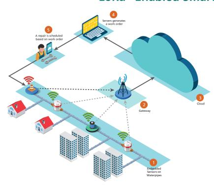
Use Case Example: Smart Water Flow Monitoring System Using LoRa
